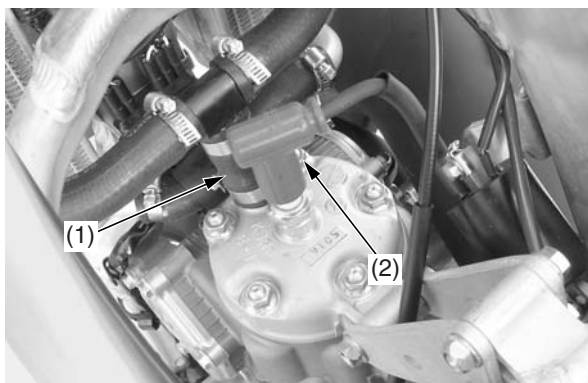
(1) water hose (2) spark plug cap
