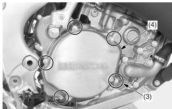
(3) clutch cover bolts (4) clutch cover
