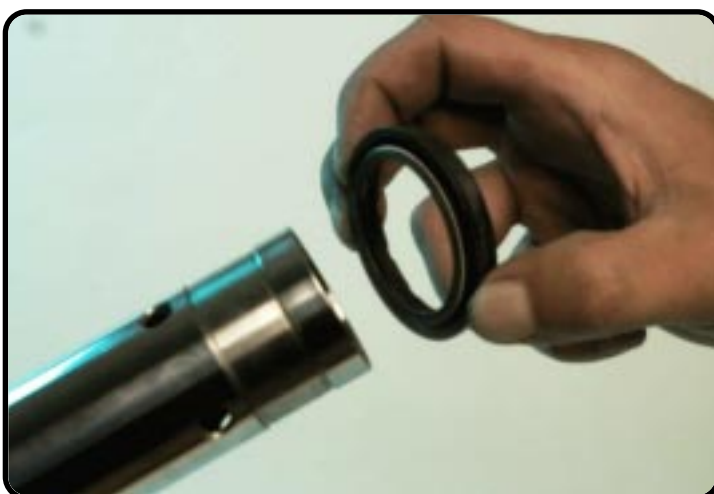
Remove the dust wiper.
