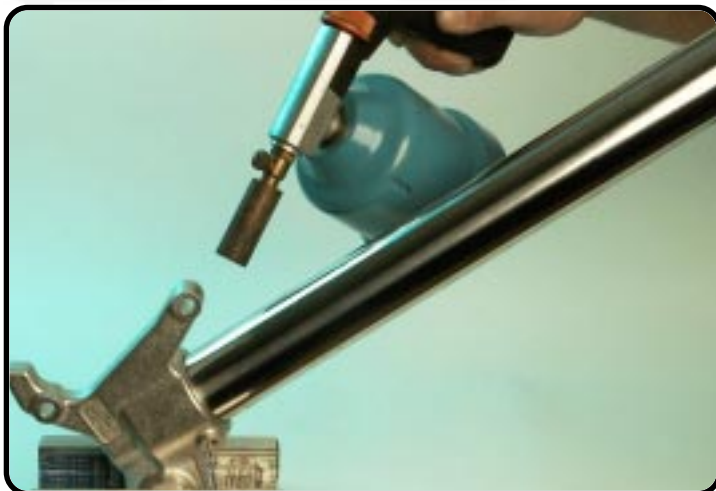
Heat the axle-clamp.
