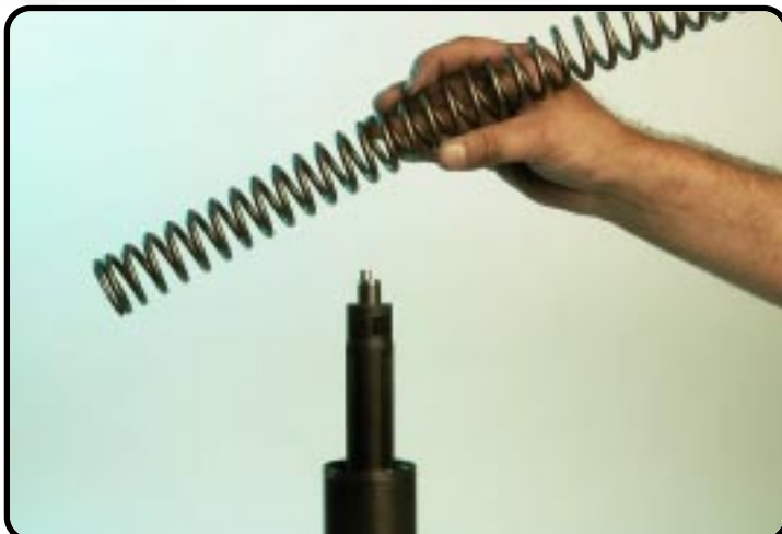
Remove the spring.
