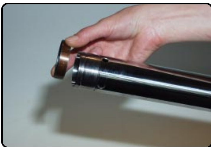
Remove DU-bush outer-tube.
