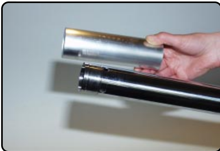
Remove DU-bush inner-tube.
